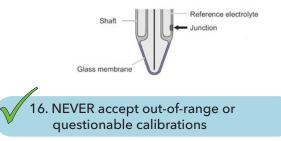
Any data collected with an electrode that has a poor calibration result will likely not be usable.
